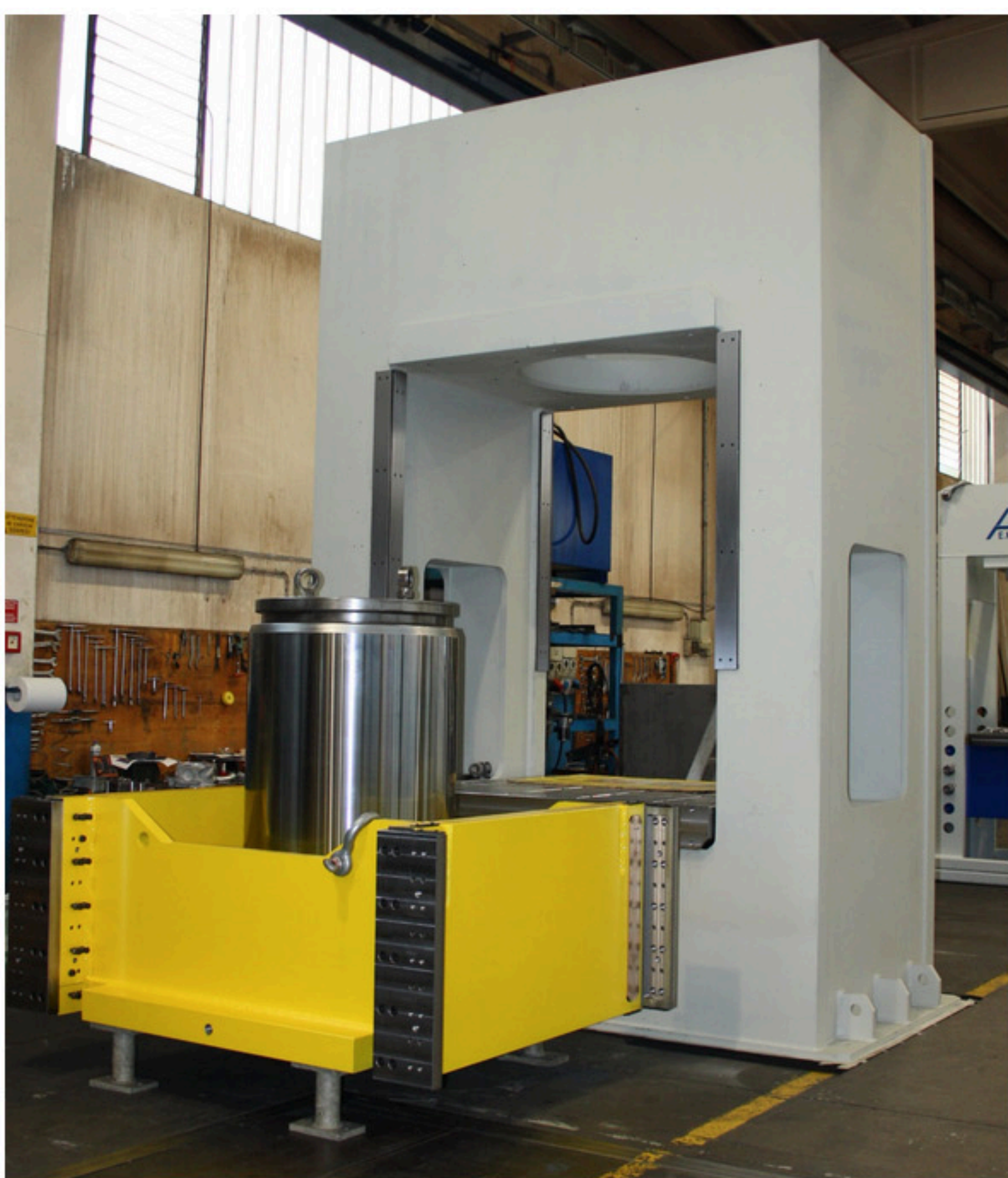
FRAME - MOBILE FLOOR AND CYLINDER READY TO ASSEMBLE
