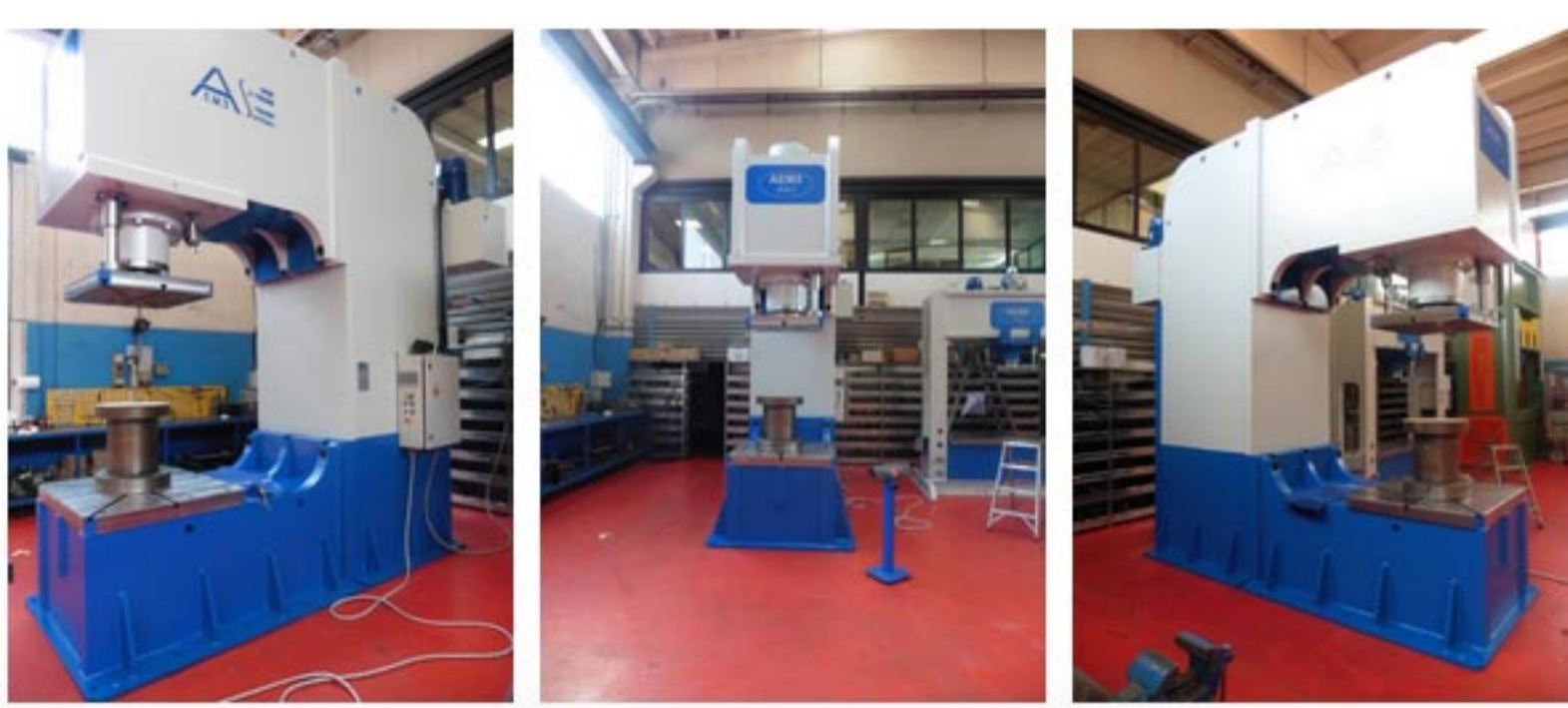
GOOSENECK PRESS POWER 200 TONS
